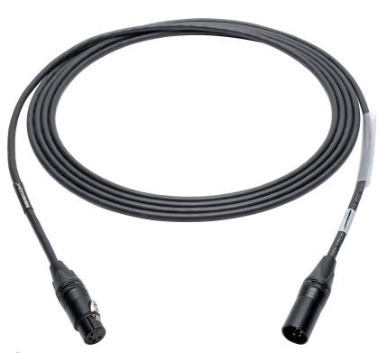
feed and a two conductor 18 AWG power feed, terminated to Neutrik NC4MXX 4-pin male and NC4FXX 4-pin female connectors. These cables can be used in conjunction with fixtures such as the Apollo MXR 2, Chroma-Q Cascade, Morpheus ColorFader and the Wybron CXI or any other power and lighting converter that utilizes a 4-pin XLR connection.
